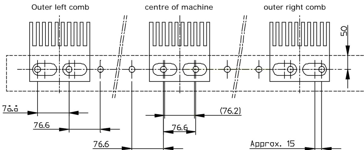
All DTS-C modules should be placed level. To ensure the DTS-Comb can slide sideways in order to follow on the thermal expansion of the belt we recommend to fit the original shouldered screws only. These screws are supplied with the combs (2 each). Do not overtighten the bolts (max. 13 Nm).
