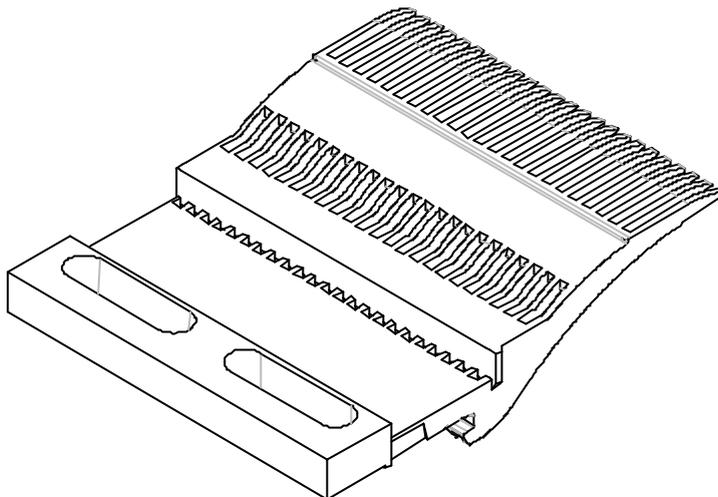
The DTS combs are equipped with oblong holes, which are centered at 76.2 (3") pitch. These oblong holes are used to bolt the combs onto the supporting profile. The supporting profile should be drilled with M6 holes at 76.6mm pitch. Using 76.6mm pitch enables the combs to accommodate thermal expansion over the full width of the machine. It is recommended to use RR2000 belts with Positrac to ensure thermal expansion is equal to both sides.
