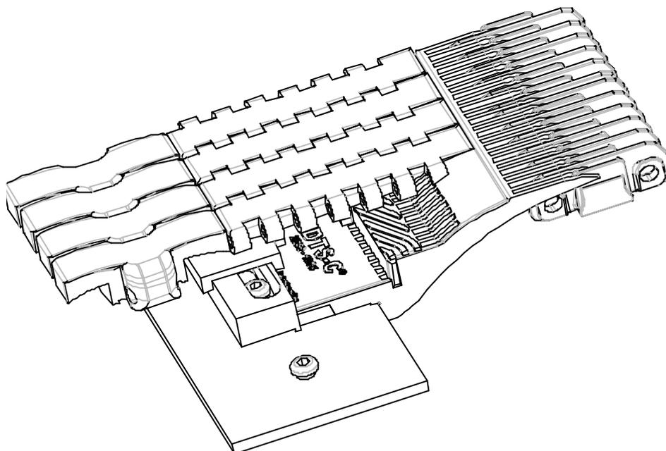
DTS-C is a brand new system which improves self-clearing of the infeed and discharge in combination with 2" Raised Rib modular belts. The system is designed for cans & PET, it can be used at the infeed of machines with glass. It is not recommended to use DTS-C at the outfeed of machines with glass. For optimum performance of the DTS-C transfer system please follow these guidelines carefully.
